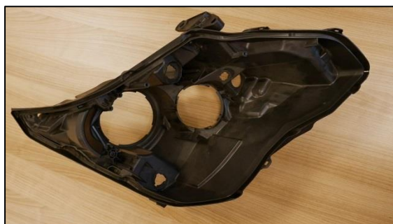
Figure 16: An automotive headlamp casing made using recycled plastic (Photo: David Jones)
